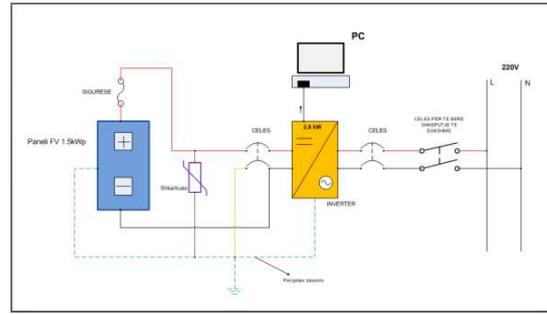
**Figure 2:** PV panel 1500Wp scheme connected with grid
